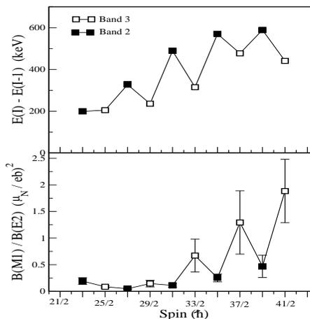
FIG. 2: The staggering in  $E(I) - E(I-1)$  and  $B(M1)/B(E2)$  for Band 2 & 3 of  $^{137}\text{Pm}$  are shown in upper and lower panel respectively.
