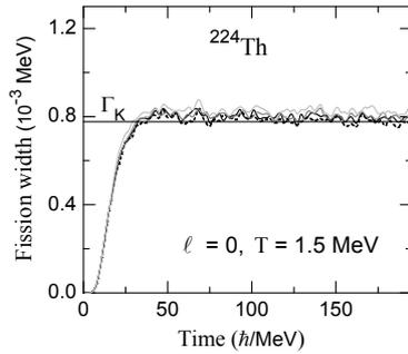
FIG. 2: Time-dependent fission widths from Langevin equations for different shapes of  $m$  as given in Fig. 1.
