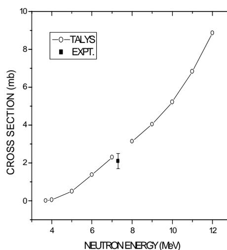
Fig.1.  $^{90}\text{Zr}$ (n,p) $^{90}\text{Y}^m$  reaction cross-section vs. neutron energy.
