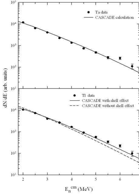
FIG. 2: Neutron evaporation spectra from  $^{208}\text{Pb}$  and  $^{184}\text{W}$ .
