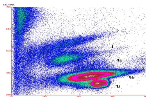
FIG. 1: PSD spectrum in one of CsI(Tl) detector in Ta target shows clear separation of various groups of particles.
