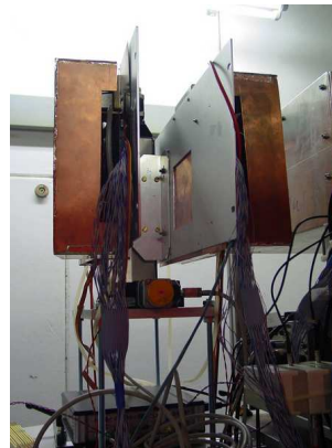
FIG. 2: GEM chambers as mounted in the beam area
