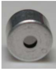
Fig.1. Piezo electric transducer used at PICASSO collaboration (upper picture) and condenser microphone (lower picture).
