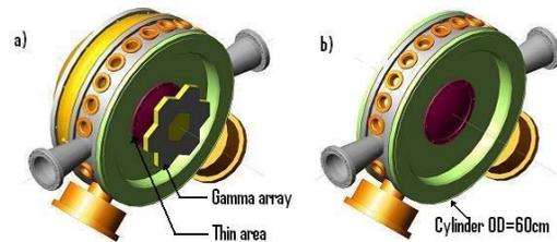
Fig.2. Schematic of hemispherical and flat configurations of the CPDA
