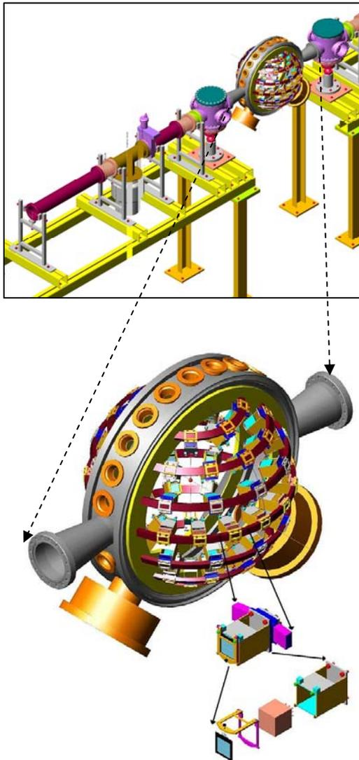
Fig. 1. Schematic of the CPDA. Expanded views of the spherical mount and the detector module are shown below.
