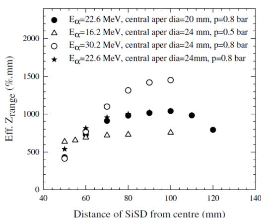
**Fig. 2** Efficiency plots as a function of distance of the SiSD from the centre of the target chamber for 3 beam energies. The pressure of the He gas and central aperture diameter are indicated.
