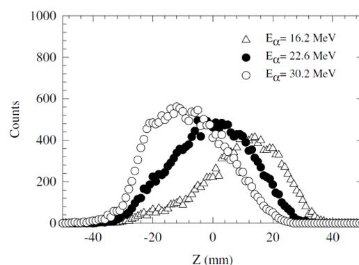
**Fig. 3** Simulation results at three alpha energies for SiSD at 70 mm from the centre showing z-region contributing to  $\alpha$ - $\alpha$  coincidences. Here a 24 mm aperture is placed at  $z=0$ .
