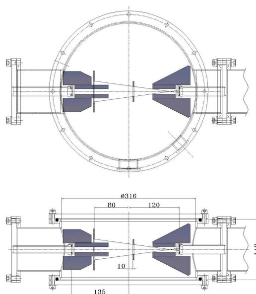
**Fig. 1** Top and side views of gas target chamber showing only the essential features.
