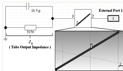
Fig. 2 Simulation of matching network in CST
