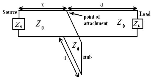
Fig. 1 Stub attached to a transmission line
