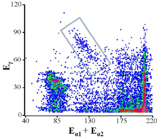
**Fig. 2** Two dimensional plot of sum energy of  $\alpha$ -particles detected in the SiSD vs sum energy of  $\gamma$ -rays detected in the BGO array (100keV/ch for both) at  $E_\alpha = 22.5$  MeV for an integrated beam charge of  $\sim 175 \mu\text{C}$ . The box indicates the region of interest (see text).
