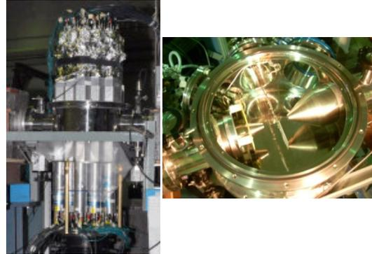
**Fig. 1** Experimental set up showing the BGO detectors (left) and gas target chamber with SiSD and heavymet shield (right).
