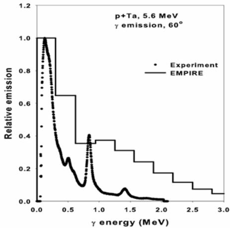
Fig. 1. Comparison of measured and calculated  $\gamma$  energy distribution in 5.6 MeV  $p + {}^{181}\text{Ta}$  at  $60^\circ$ .
