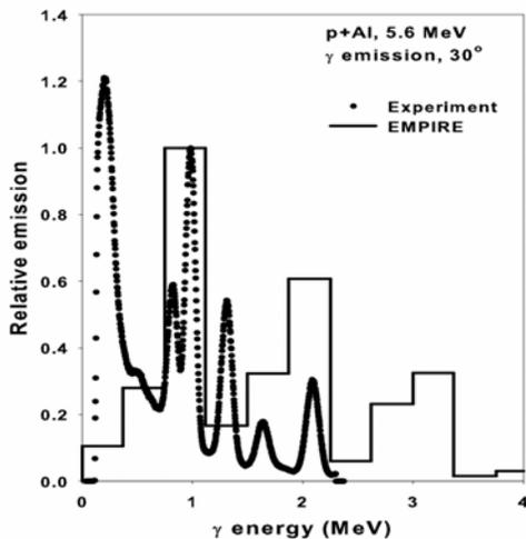
Fig 2. Comparison of measured and calculated  $\gamma$  energy distribution in 5.6 MeV  $p + \text{Al}$  at  $30^\circ$ .
