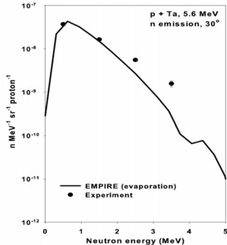
Fig.3. Measured and calculated energy distribution of neutrons in 5.6 MeV  $p + {}^{181}\text{Ta}$  at  $30^\circ$ .
