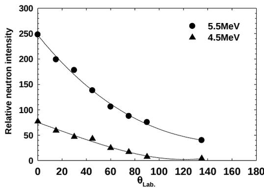
**Fig. 3** Angular distribution of neutron yield from thick Lithium target from 4.5 and 5.5 MeV proton energies. The statistical error in the data is less than 0.1%.
