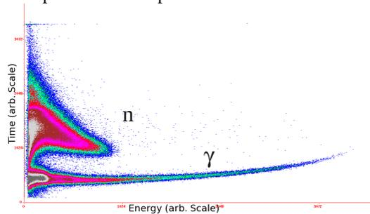
**Fig. 2** Neutron gamma 2-D spectrum from 5.5 MeV proton beam interacting with thick lithium target.
