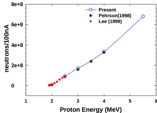
**Fig. 1** Neutron yield from a 5mm thick natural Lithium target for proton energies from 2.5 to 5.5 MeV. The other experimental data [1, 2] are also plotted for comparison.
