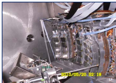
Figure 1: HiRA set up with 20 telescopes inside the S800 scattering chamber.
