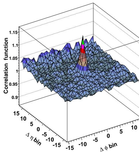
FIG. 1: 2-D plots of correlation function between PMD clusters and FTPC tracks for STAR CuCu  $\sqrt{s_{NN}}=200 \text{ GeV}$  data.  $\Delta(\eta)$  bins=0.023,  $\Delta(\phi)$  bins=0.15 rad.
