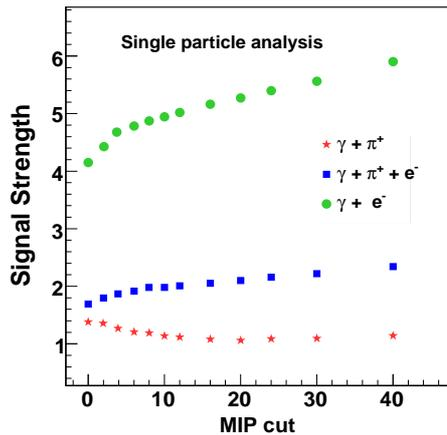
FIG. 3: Variation of the *signal strength* for single particle GEANT simulation
