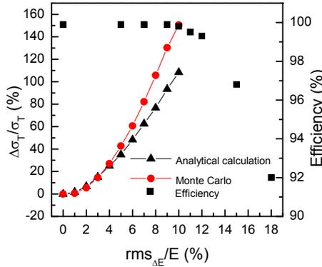
FIG. 2: The variation of efficiency as well as time resolution of the timing RPC due to the variation in electric field, arises due to the non-uniformity of the surface of the RPC electrodes.
