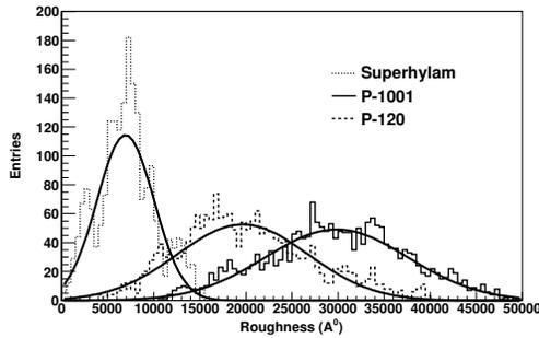
FIG. 1: The surface roughness profile of three different grade bakelites.
