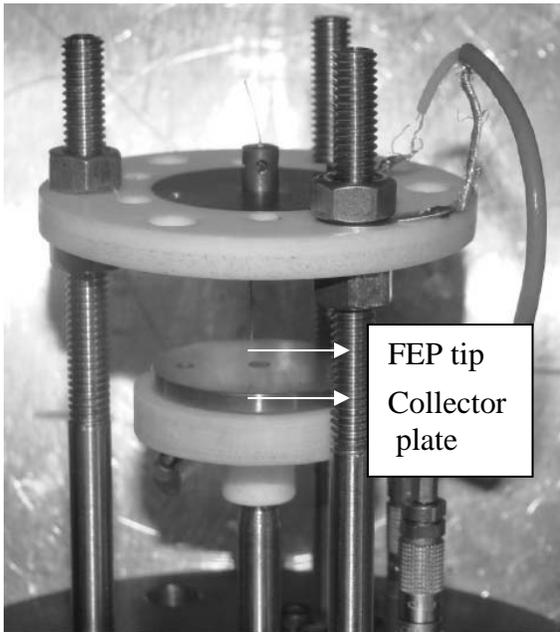
**Fig. 2** Setup for FEP probe study
