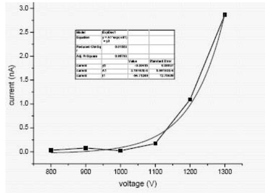
**Fig. 3** V-I characteristic of a FEP probe
