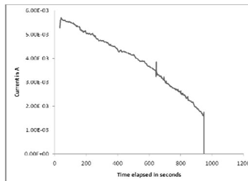
Fig. 1 Current flow through etching system
