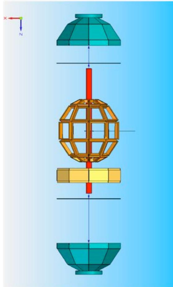
**Fig. 4** One of the proposed mechanical designs of HYDE detector for FAIR. The vacuum vessel is divided in 3 parts to help operation and maintenance. The inner structure holds 54 detector cells, where DSSSD detectors of high granularity are mounted.
