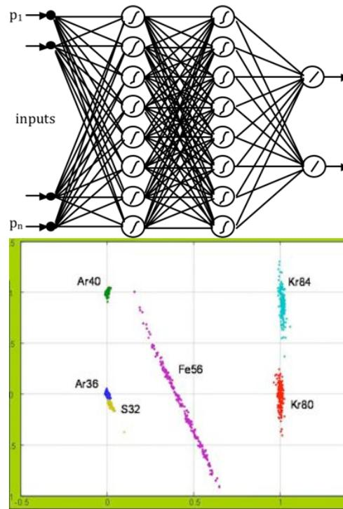
**Fig. 2** Up: Simple neural network architecture. Down: Classification of pulses of several heavy ions impinging on NTD silicon detector. See text for details.
