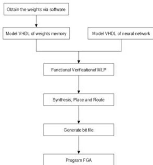
**Fig. 3** Flow diagram for ANN implementation in an FPGA dedicated to DPSA. See text for details.
