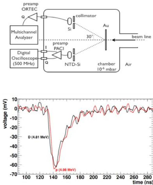
**Fig. 1** Up: Experimental setup for DPSA studies. Down: Typical pulse shapes for low energy protons and deuterons.
