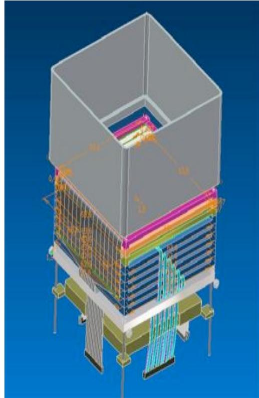
**Fig. 5** Prototype of detection cell of the HYDE detector. The pink, orange, green and blue layers correspond to 40  $\mu\text{m}$ , 100  $\mu\text{m}$ , 500  $\mu\text{m}$  and 1500  $\mu\text{m}$  DSSSD detectors, respectively. The grey box on the top is foreseen to protect the silicon layers when manipulating the detector cell.
