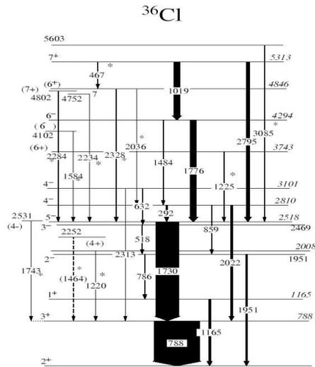
FIG. 3: Partial level scheme for  $^{36}\text{Cl}$  observed in the present work. The new gammas found are marked by asterisk.
