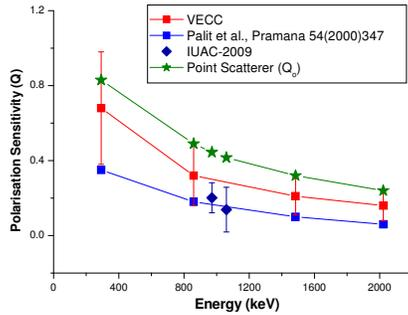
FIG. 1: The polarisation sensitivity of a Clover detector in different implementations of INGA. See text for detail.
