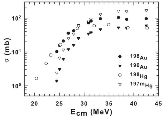
FIG. 2: Measured excitation function for d capture ( ${}^{197m,198}\text{Hg}$ ) and neutron transfer ( ${}^{196,198}\text{Au}$ ) in  ${}^6\text{Li}+{}^{197}\text{Au}$  reaction.
