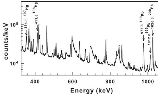
FIG. 1: Gamma ray add back spectrum of the whole array at 45 MeV for  ${}^7\text{Li}+{}^{197}\text{Au}$  reaction
