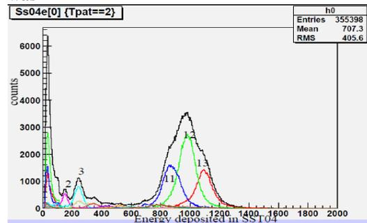
**Fig. 3** Charge identification from deposited energy.
