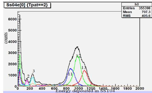
**Fig. 3** Charge identification from deposited energy.
