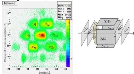
**Fig. 1** (left) Incoming particle ID plot (right) Diagram showing the SSTs around the target.
