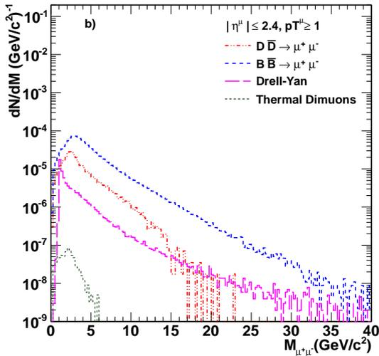
FIG. 2: Relative invariant mass distributions of decay muons from thermal, open beauty, open charm and Drell-Yan at  $\sqrt{s_{NN}} = 2.76 \text{ TeV}$ , inside CMS detector ( $|\eta^\mu| \leq 2.4$ ).
