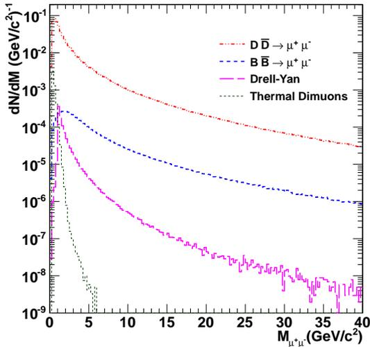
FIG. 1: Relative invariant mass distributions of decay muons from thermal, open beauty, open charm and Drell-Yan at  $\sqrt{s_{NN}} = 2.76 \text{ TeV}$ .
