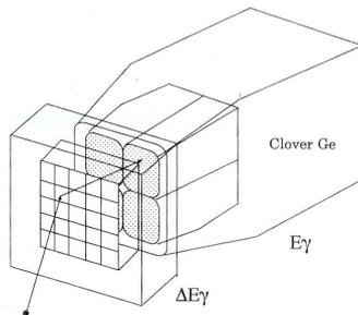
FIG. 3: The HPGe clover & Planar configuration, showing a prototype planar detector in front of the Clover detector [2].
