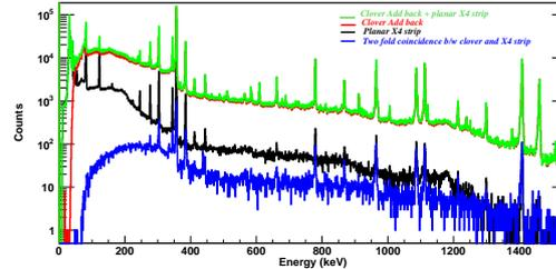
FIG. 4: Black: The X4 planar strip spectrum. Red: Clover add-back spectrum. Green: Sum spectrum of coincident events in the clover and X4 strip. Blue: 2-fold coincidence spectrum between clover addback and planar X4 strip.
