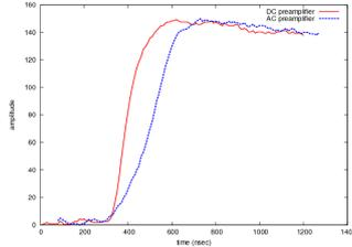
FIG. 2: Preamplifier pulses from DC and AC strips stored in the Pixie-16 module.
