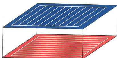
FIG. 1: Schematic diagram of the 10X - 10Y double sided Ge strip detector.
