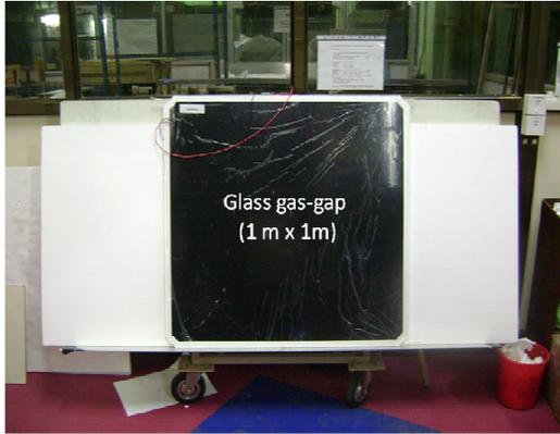
**Fig. 1** A typical glass gas-gap (1m x 1m) with graphite coating to be configured into an RPC for muon tomography
