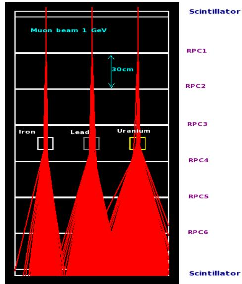
**Fig. 2** GEANT-4 simulations of the Muon Tomography system for a normal incident monoenergetic stream of muons
