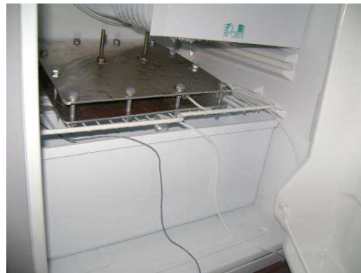
Fig. 3 The condenser cum saturator inside the refrigerator maintained at 9^{\circ}\text{C}
