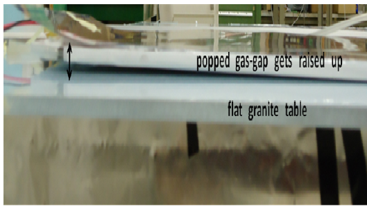
Fig. 2, A gas-gap with a popped spacer gets raised up on a flat granite table
