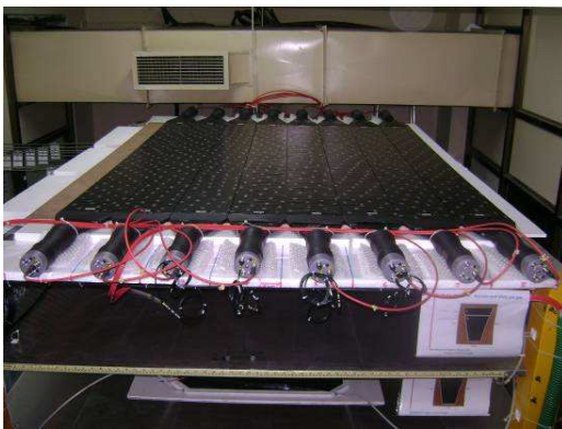
Fig. 2 The eight scintillators in the top layer (shelf # 9 : C91D91 to C98D98) of the cosmic rack with PMTs at both the ends
