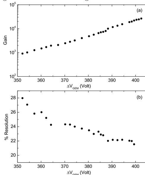
FIG. 2: (a) Effective gain curve of the triple GEM, operated in argon/ $CO_2$  70/30. (b) Energy resolution as a function of  $\Delta V_{GEM}$ .
