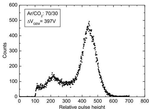
FIG. 1: (Pulse height distribution for 5.9 keV  $Fe^{55}$  source obtained with triple GEM detector.
