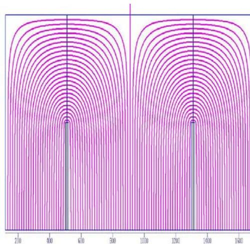
Fig.2. Field lines with coil slots 8 m separated.
