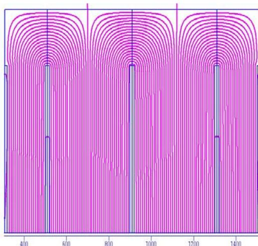
Fig.3. Field lines with coil slots 4m separated.
