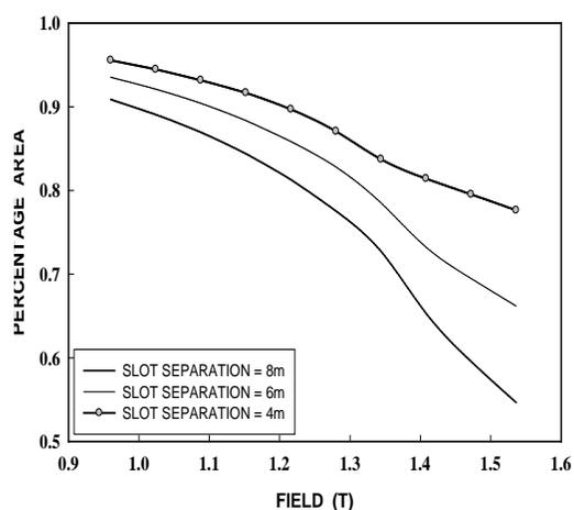
Fig.4. Improvement in field uniformity with slots separated by small distance.
