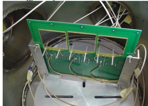
Fig.4: Three resistive anode detectors
