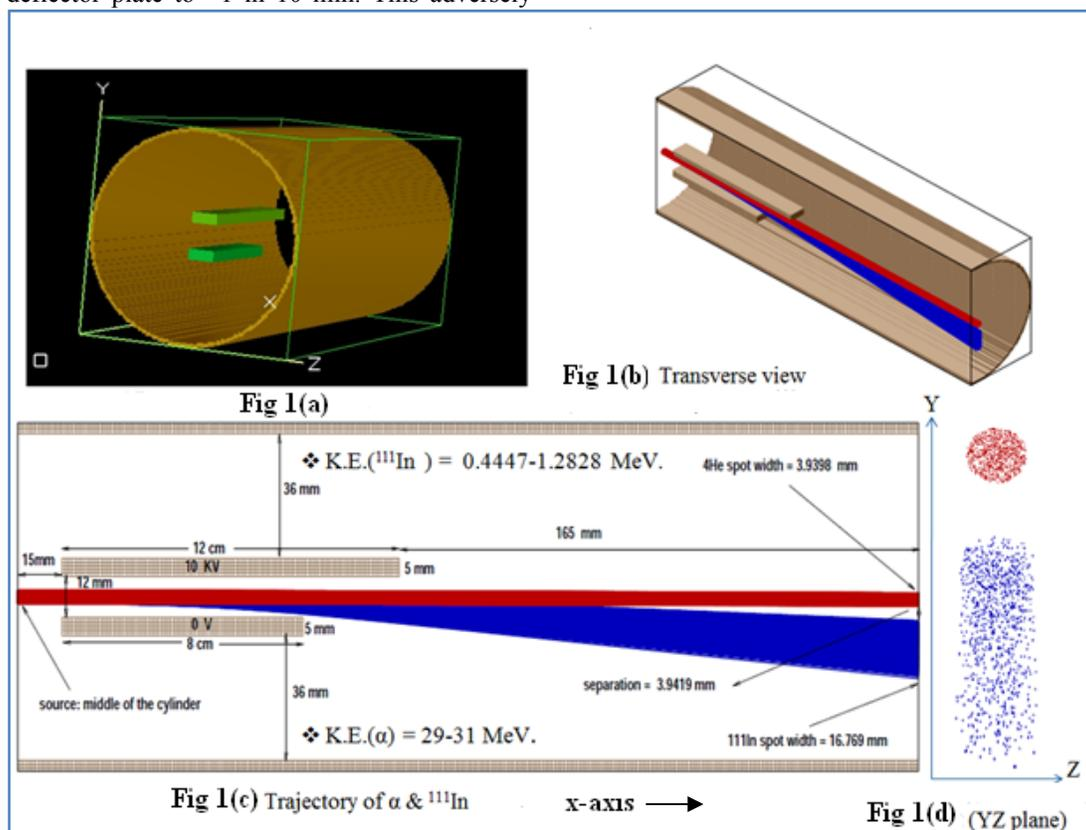
Fig 1. Design of Electrostatic deflector and ion trajectory of recoil  $^{111}\text{In}$  and primary alpha beam
