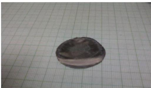
**Fig. 5**  $^{116}\text{Cd}$  foil of thickness  $\sim 3.0 \text{ mg/cm}^2$
