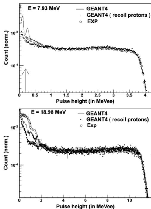
FIG. 1: Comparison of experimental and GEANT4 simulated pulse height spectra for neutron energies 7.93 and 18.98 MeV. Here line shows GEANT4 simulation considering all reaction process and dot shows recoil proton only. Detector thresholds are shown by arrows.
