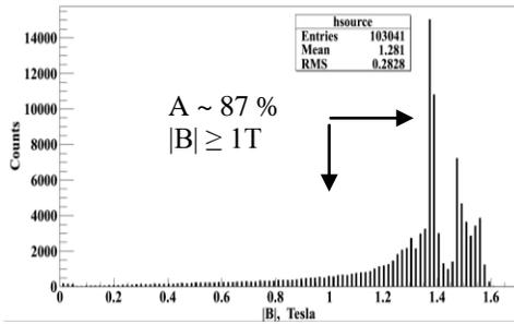
**Fig. 3** Distribution of  $|B|$  in area of  $16\text{ m} \times 16\text{ m}$  for standard configuration.
