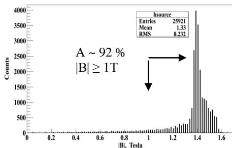
**Fig. 5** Distribution of  $|B|$  in area of  $16\text{ m} \times 16\text{ m}$  for nonstandard configuration.
