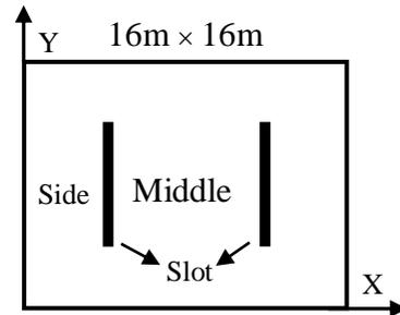
Fig. 1 Schematic of ICAL magnet
