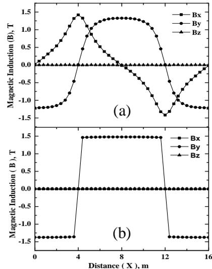
Fig. 2 Magnetic induction variation with distance at total current of 60 kA-turns, (a)  $Y = 3$ m,  $Z = 0$ m, (b)  $Y = 8$  m,  $Z = 0$ m using  $L_S = 8$ m.
