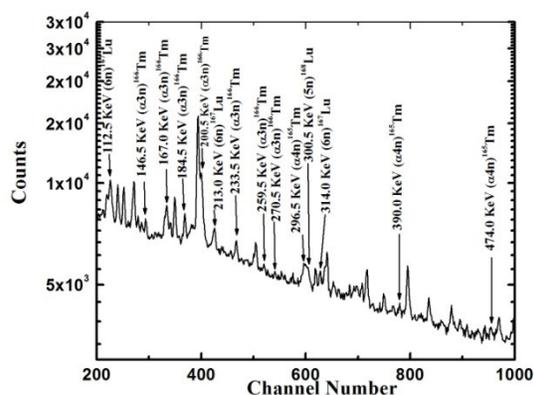
**Fig. 2** Gamma ray energy spectra observed from  $^{19}\text{F} + ^{154}\text{Sm}$  system at 100MeV.
