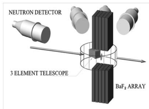
**Fig.1** A typical experimental setup
