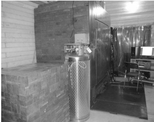
FIG. 3: PCGe detector with moderate passive shielding material.
