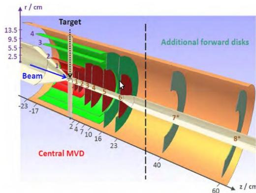
Fig.2 Micro Vertex Detector with lambda disks
