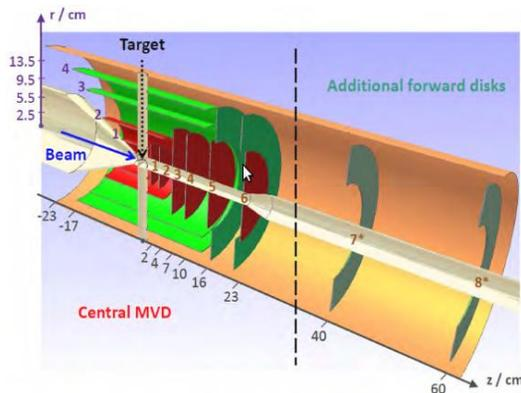
Fig.2 Micro Vertex Detector with lambda disks
