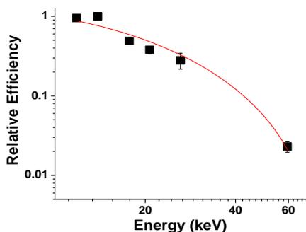
**Fig. 2** Efficiency of Si-PIN detector
