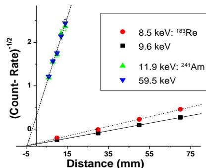
**Fig. 3** Measurement of the position of the Si crystal.
