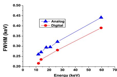
**Fig.1** Comparison of variation in FWHM with photon energy for analogue and digital pulse processing.
