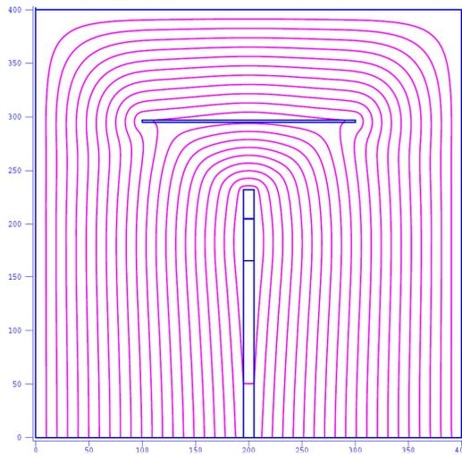
Fig.3. Field lines with an extra air slot.
