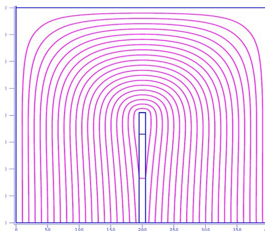
Fig.2. Field lines in a quarter of a magnet plate with no extra slot
