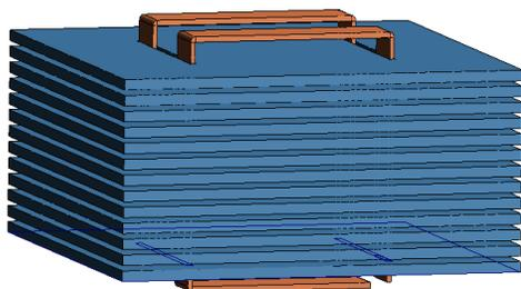
Fig.1. INO prototype magnet with a few layers (schematic) showing coils
