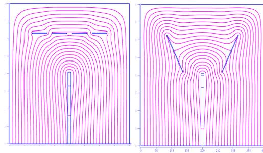
Fig.5. Field lines with various types of air slots.
