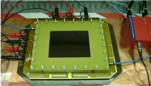
Fig.3 Photograph of assembled GEM detector.
