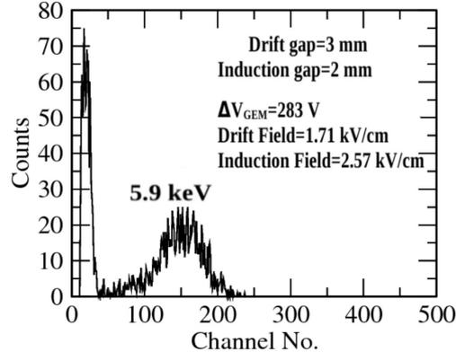
Fig.4 X-ray pulse height spectrum obtained with Single-GEM detector for P-10 gas.
