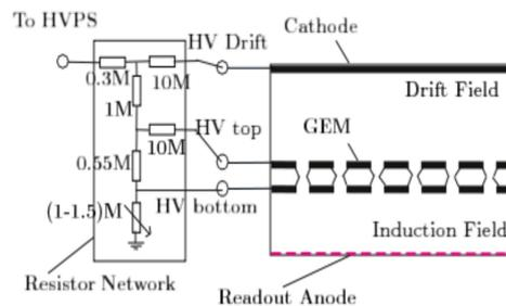
Fig.2 Schematic of single GEM detector with resistor network.
