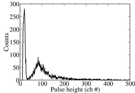
Fig.5 Beta energy loss spectrum from a <sup>90</sup>Sr source obtained with Single-GEM detector for P-10 gas.
