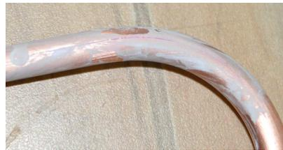
Fig. 2, DP Test showing cracked line on tube
