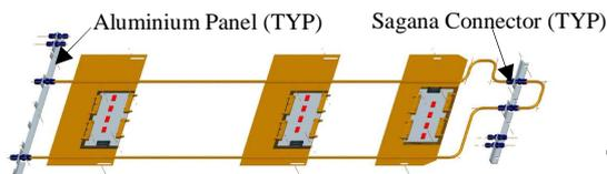
Fig. 1, Cu cooling circuit for a typical CMS-RPC
