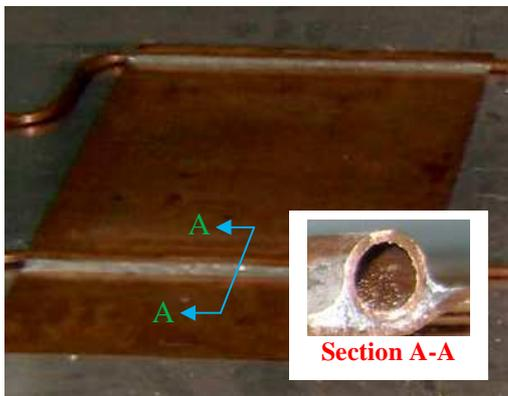
Fig. 4, Cooling ring after successful soldering
