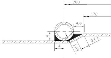
Fig. 3, A typical soldering joint detail
