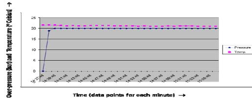
Fig. 6, Leak rate of Cu cooling circuit at 20 bar of Argon gas pressure
