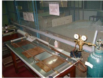
Fig. 5, Cu cooling circuit after fabrication under leak test with 20 bar pressure of Argon gas
