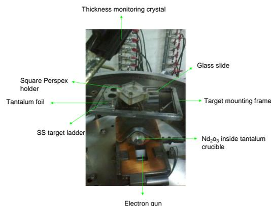
**Fig. IV** Mounting arrangements in the E-beam deposition unit at IUAC
