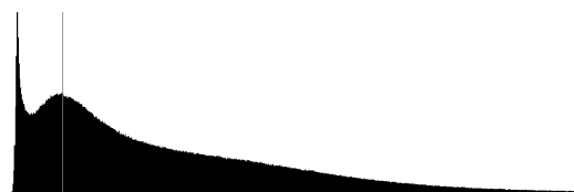
Fig.4 Beta spectrum of Sr-90 with ANUSANSKAR ASIC coupled with PAD detector
