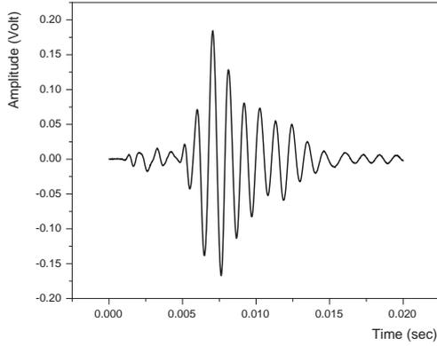
FIG. 2: Typical signal by microphone after passing through 150 Hz high-pass filter.
