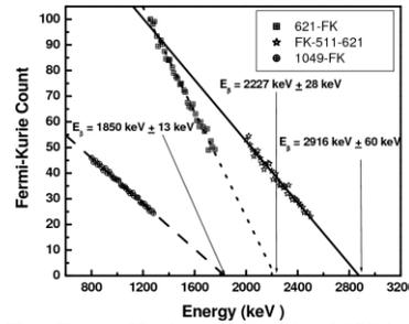
Figure 2: The Fermi-Kurie plot for the 3050 keV and 2410 keV  $\beta$  decay of  $^{106}\text{Rh}$
