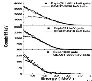
Figure 1: The beta spectrum obtained for  $^{106}\text{Rh}$  decay from the LEPS detector and compared with the GEANT simulation
