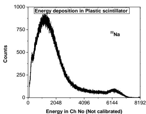
Fig 3: Energy deposition using <sup>22</sup>Na source
