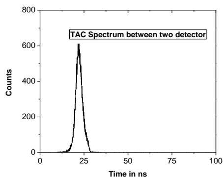
Fig 4: Time to amplitude converter peak using coincidence between two plastic scintillator where also <sup>22</sup>Na was used.
