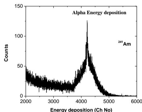
Fig 5: Energy deposition spectrum using <sup>241</sup>Am (5.38, 5.44, 5.48 MeV alpha)
