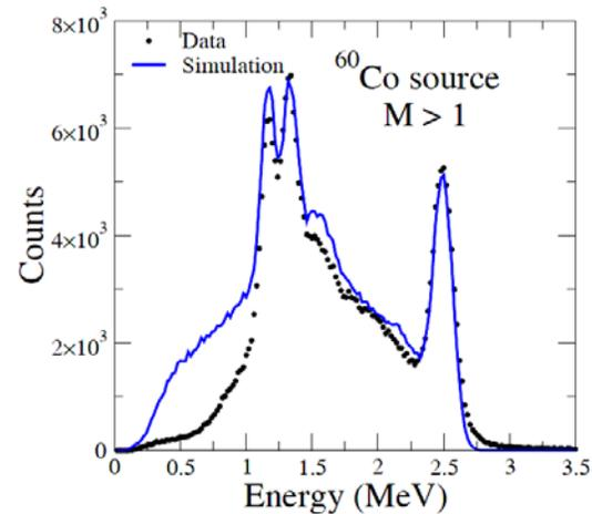
Fig. 5: Simulated spectrum (solid line) of <sup>60</sup>Co along with the experimental data (solid circle). Both are for multiplicity  $M > 1$ .
