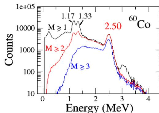
Fig.3: Sum spectrum of <sup>60</sup>Co source obtained from the TAS array for different multiplicity (M) condition.
