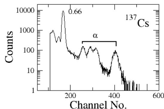
Fig.2: Raw spectrum of <sup>137</sup>Cs source obtained from a single BaF<sub>2</sub> detector.
