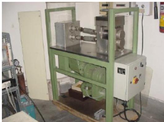
FIG. 1: Rolling machine used for the target preparation.
