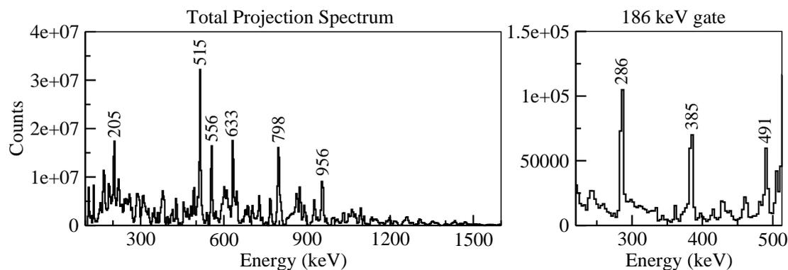
FIG. 1: Left panel: Total projection spectrum prepared from the  $E_\gamma - E_\gamma - E_\gamma$  cube, Right panel: 186 keV gated spectrum showing the coincident  $\Delta I = 1$  transitions.
