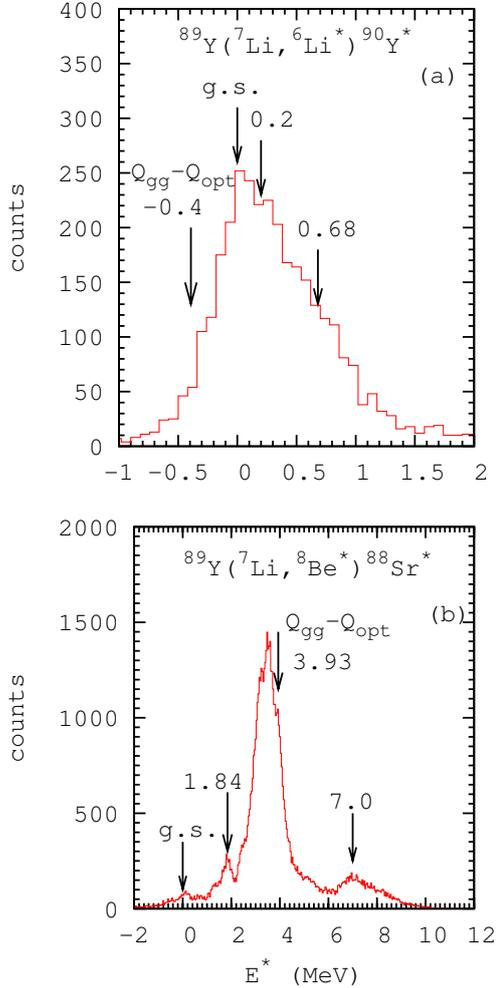
FIG. 1: Measured excitation energy spectrum of target like product for  ${}^7\text{Li}+{}^{89}\text{Y}$  reaction at beam energy 23 MeV. (a)  ${}^{90}\text{Y}^*$  in 1n-stripping reaction and (b)  ${}^{88}\text{Sr}^*$  in 1p-pickup reaction.
